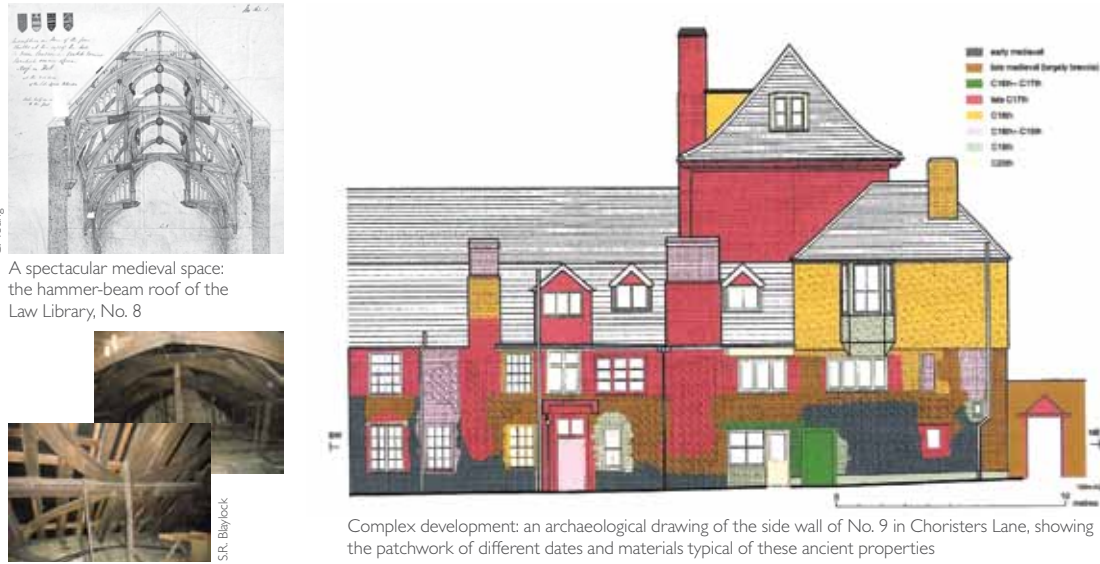
A spectacular medieval space: the hammer-beam roof of the Law Library, No. 8. Complex development: an archaeological drawing of the side wall of No. 9 in Choristers Lane, showing the patchwork of different dates and materials typical of these ancient properties.
